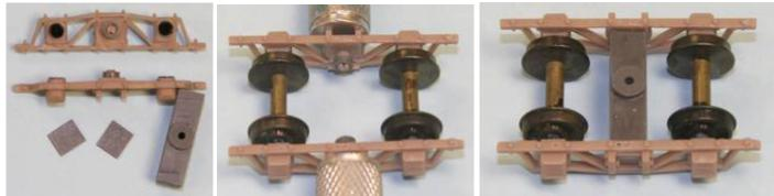
**Step 3:** (Center & right photo) Insert the wheels and hold in place with X-Acto® knife handles or similar. Drop the bolster over the pins. There should be <u>no</u> side-to-side "slop" between the bolster and pin retainer ring, only enough to allow rotation around the pin. Press the ring closer to the back of the sideframe to tighten the fit and test again. Once satisfied, put a small drop of CA on the pin to lock the ring in place.
