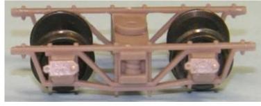
At left is the completed, unpainted "common" style truck; inprocess photos show the "swing motion" style. Together, these represent nearly all freight car applications by Maine two-foot gauge railroads. Each truck kit is composed of cast urethane side frames, bolster, a sheet of details, Kadee HOn3 insulated wheels and #0-48 x ¼" screws.
